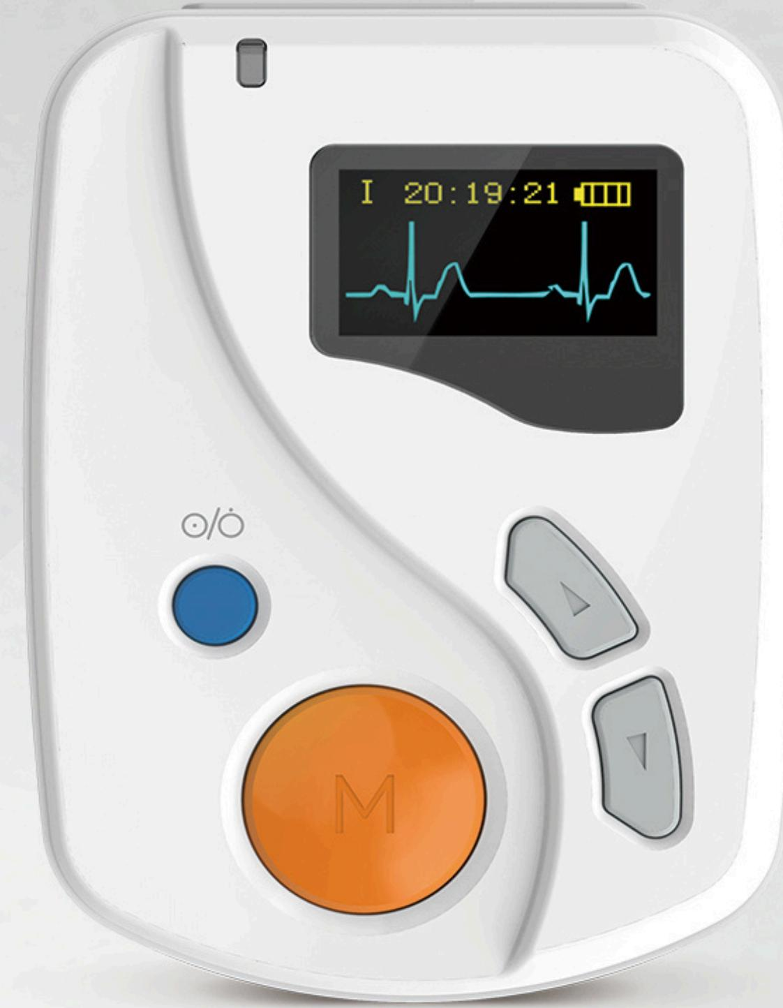
Dynamic ECG Systems adopt 12-lead system of international standard, which can continuously record ECG waveform for 24-hour and analyze ECG waveform by the PC software. It is applicable for use in medical institution and community.
